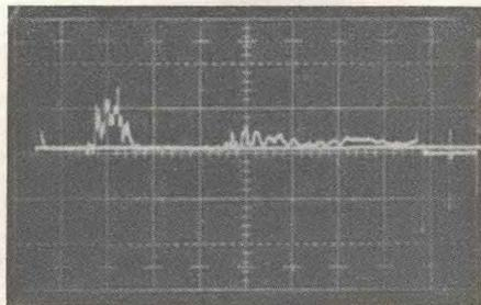
Fig. 5. Cavity gas-pressure instrumentation gage signal from alcove 4: 100-kpsi-range Norwood gage, 2 msec/cm, 25 kpsi/cm.
